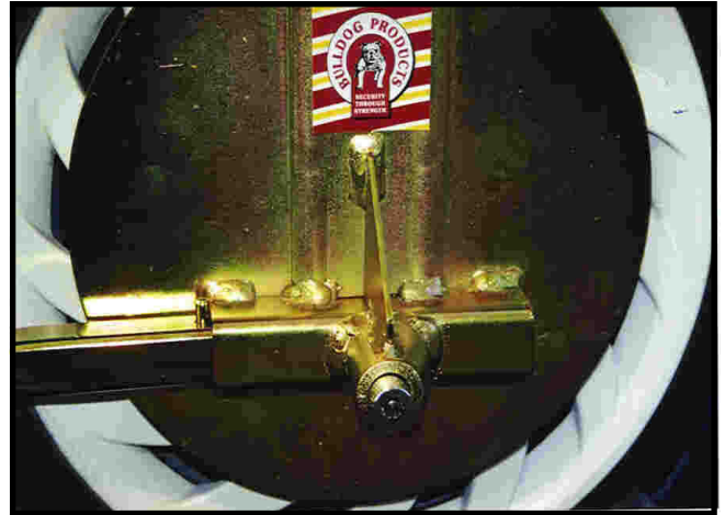
2. Fit left hand arm into channel until roll pin touches channel.
