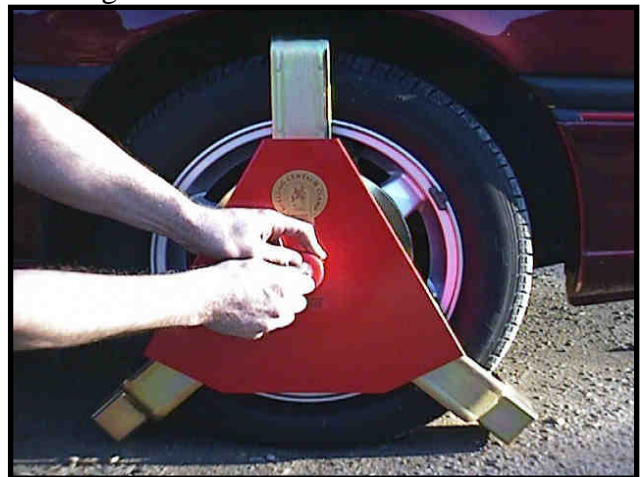
11. Press thumb against red cap, push in key and rotate 1/4 turn anti-clockwise to UNLOCK. Now place cover plate (part No.11) so that lock engages with hollow nut and rotate key 1/4 turn clockwise to LOCK and release key.
