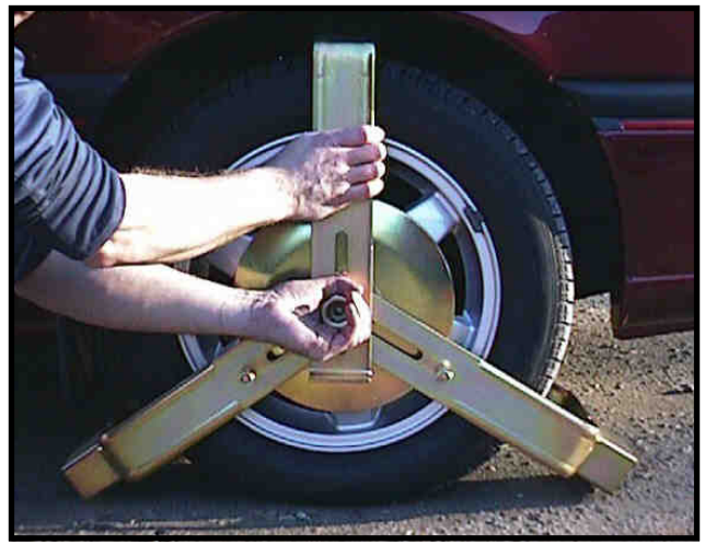
7. Still holding nut with left hand, swing round top arm to vertical position.
